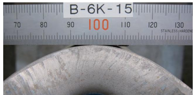
(g) High Tensile Steel with grinding /  $t=20.1$  / Elongation=24
