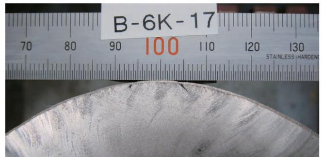
(h) High Tensile Steel with grinding /  $t=23.1$  / Elongation=26
