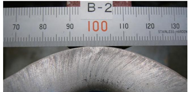
(e) Mild Steel with grinding /  $t=17.8$  / Elongation=32
